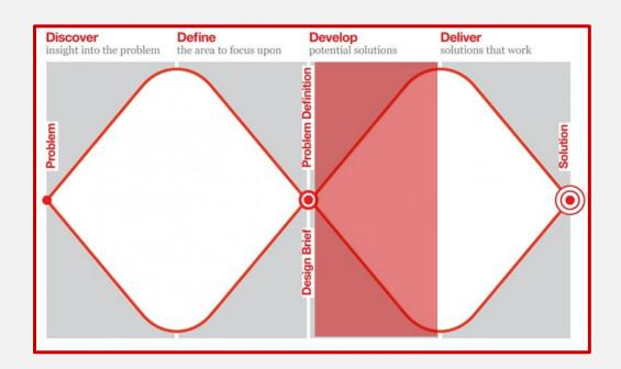
The third quarter marks a period of development where solutions are created, prototyped, tested and iterated. This process of trial and error helps designers to improve and refine their ideas.
