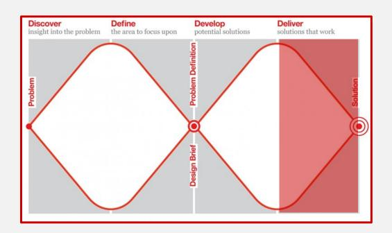
The final quarter of the double diamond model is the Deliver phase, where the resulting product or service is finalised and launched.
