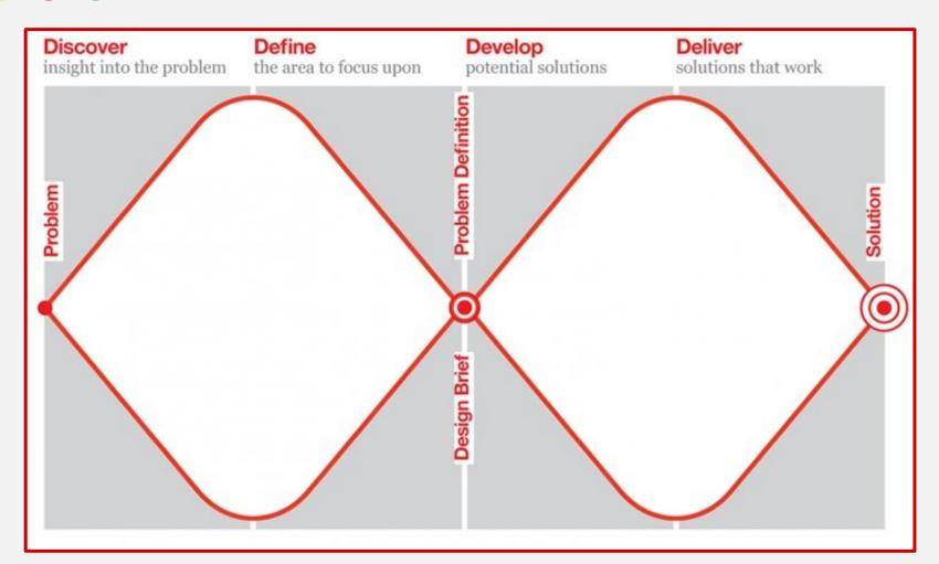
Divided into four distinct phases – Discover, Define, Develop and Deliver – the Double Diamond is a simple visual map of the design process.
